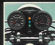
Integrated instrument panel with big instruments and signals in centre.
