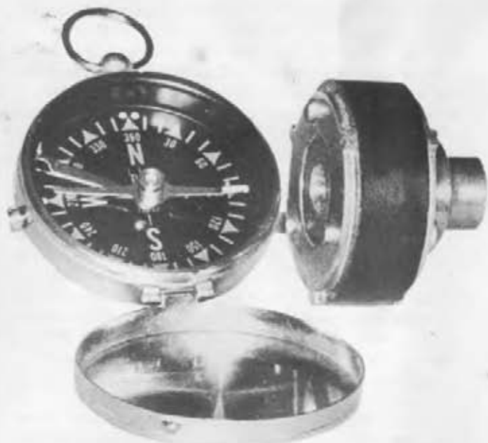
To check for a reversed magnet in the signal rotor, hold a compass near the rotor, then move it around the face of the rotor. If the needle swings around end-for-end, it indicates a reversed magnet.
