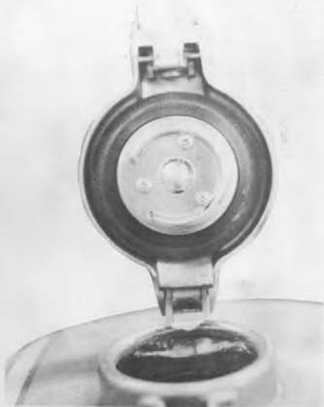
The vent on the locking-type cap leads to a serpentine passage. Suck on the vent to check it. This cap is used on all 1972 models.
