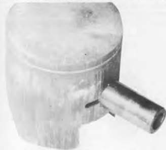
This piston shows uncontrolled blow-by caused by sticking of both piston rings. This is caused by the use of incorrect oil, which allows hard carbon or lead deposits to form in the ring grooves. Note the scoring caused by piston seizure. This results from the hot gases destroying the oil film, and this reduced the heat transfer path from the piston to the cylinder wall. This piston's skirt was broken because the rider continued to run the engine in spite of seizure. The piston pin has seized in the piston because of the extreme heat caused by this abusive treatment.
