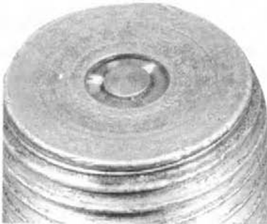
Concentrated arc. The multicolored appearance is a normal condition, caused by electrical energy consistently following the same firing path. The arc path will generally change with deposit conductivity and gap erosion. This spark plug does not need to be replaced.
