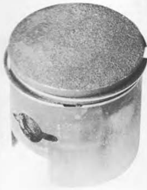
This H1 piston shows excessive blow-by past the piston rings, which have been overheated and lost tension. Note the small gap of the ring, which is an indication of lost ring tension.
