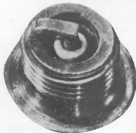
This spark plug has the correct heat range. The center electrode insulator is light tan to brown in color.
