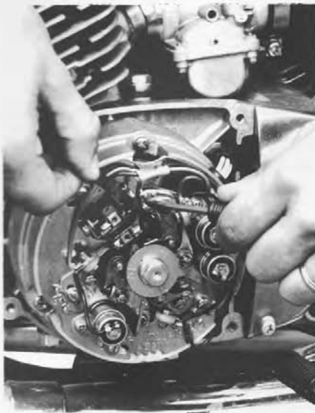
To adjust the point gap on an H1B, loosen the screw that holds the point set to the timing plate, then shift the points using a screwdriver inserted into the notch in the point set and between the dimples on the timing plate.
