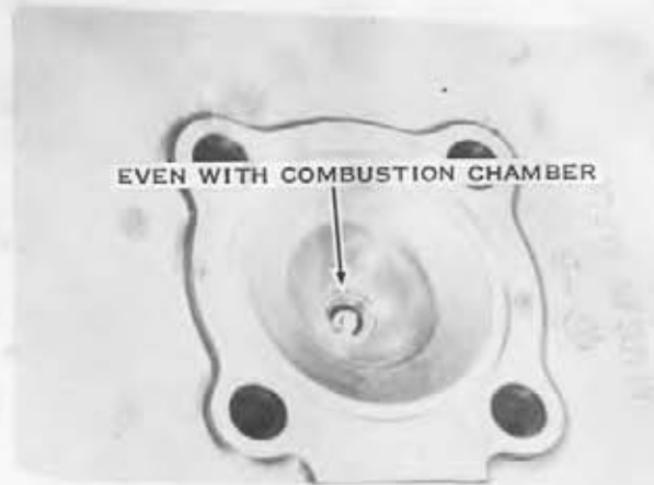
This shows the correct plug reach. All models use a \frac{1}{2} " plug reach. Be sure to use the right plugs.
