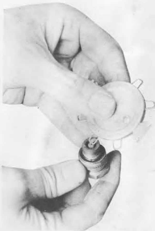
Measure the spark plug gap with only a wire-type gauge. A flat feeler gauge will give an inaccurate reading because the inside of the side electrode is not flat.
