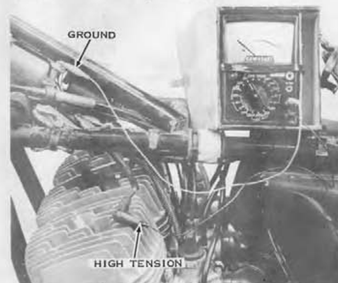
For the second coil test, connect the ohmmeter leads to the high-tension lead and to the black ground wire. There should be about 1 ohm of resistance.
