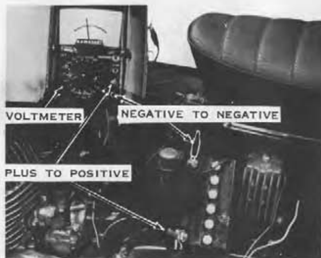
Testing the H1 battery voltage with a 30-volt DC voltmeter. It should be 12.5 volts with no load, and should not drop below 11.5 volts with the ignition and lights turned on.
