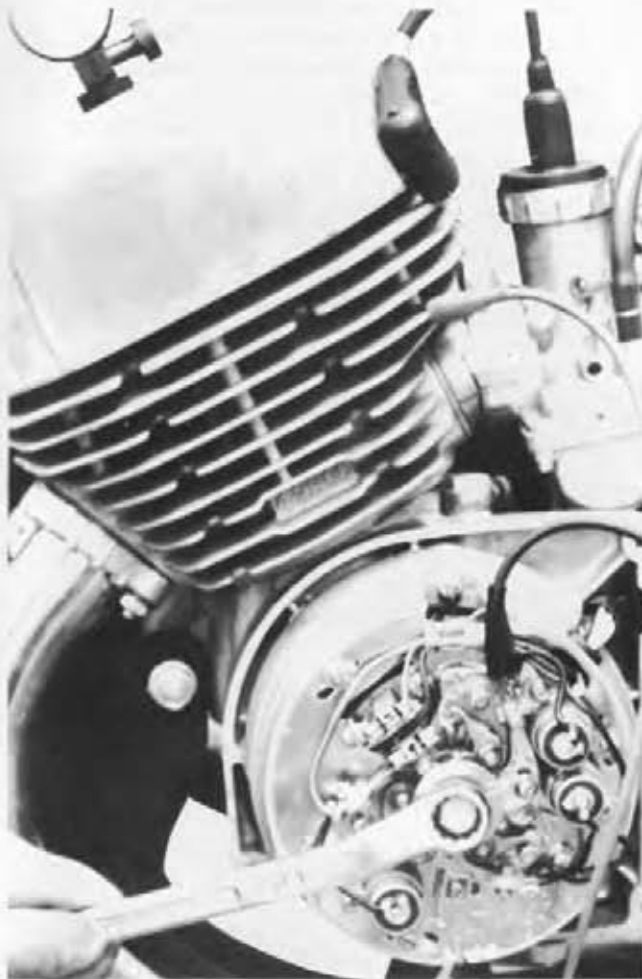
When timing the H1B ignition with a dial gauge, be sure to time the top point set first. It is mounted directly on the stator plate; therefore, changing its timing also changes the timing of the other two sets.
