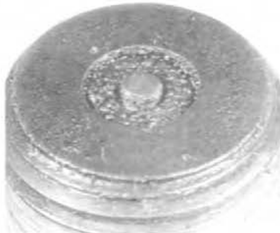
Cold-foul spark plug. These wet fuel/oil deposits can be caused by "drowning" the spark plug with raw fuel during cranking, an excessively rich fuel/air mixture, or a weak ignition system.
