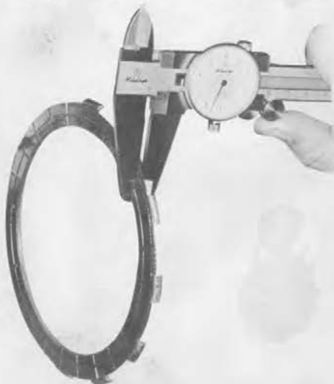
Measure the friction plate thickness. If it is less than the service limit given at the end of this chapter, the clutch will slip on acceleration.
