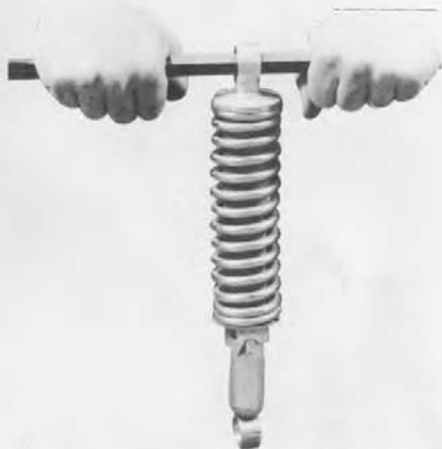
Check the rebound dampening action by inserting a rod through the top eye and compressing the shock absorber. If it springs back with a snap, the damper unit is defective; replace the shock absorber. Make sure the damper cylinder is in the as-installed position during this test or the damper valve will be drained of oil.
