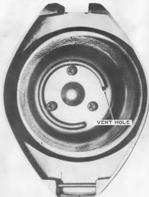
The flip-type cap is used on 1973 and later models. It is vented in the same manner as the locking gas cap.
