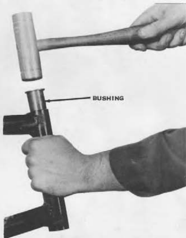
Install new swingarm bushings by heating the pivot tube with hot water, then driving the bushing in with a soft-face hammer.
