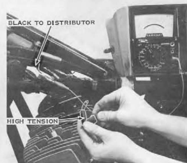
For the fourth coil test, connect the ohmmeter leads to the high-tension lead and to the black wire that normally goes to the distributor. There should be infinite resistance.
