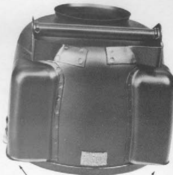
ADDITIONAL AIR INTAKES
