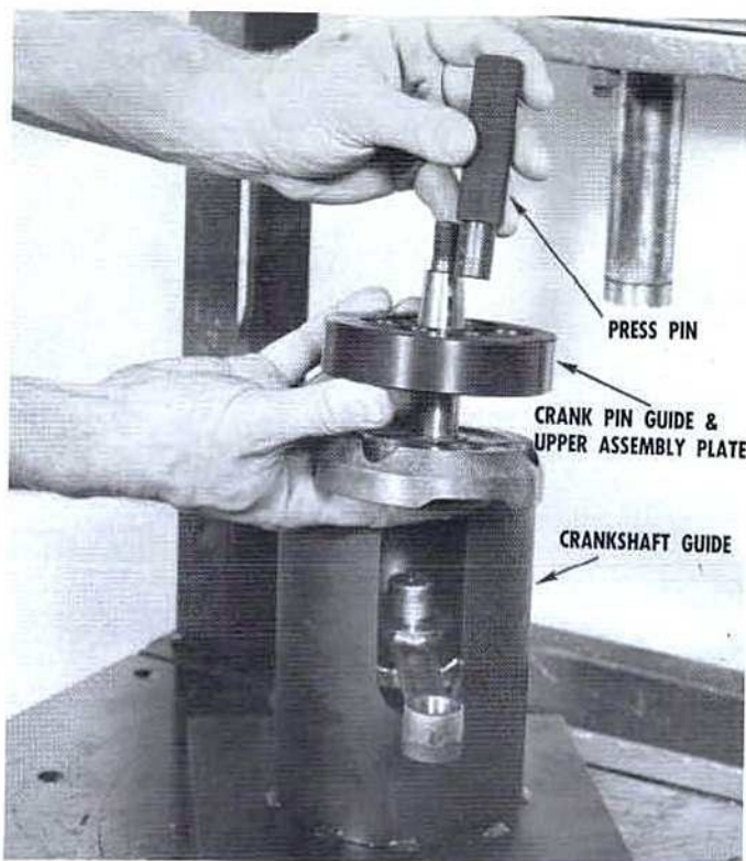
7 Place the left hand crankshaft in the upper assembly plate (tool G) as shown. Position the left hand crankshaft and upper assembly plate in the crankshaft guide, with crank pin hole in position over the crank pin.
