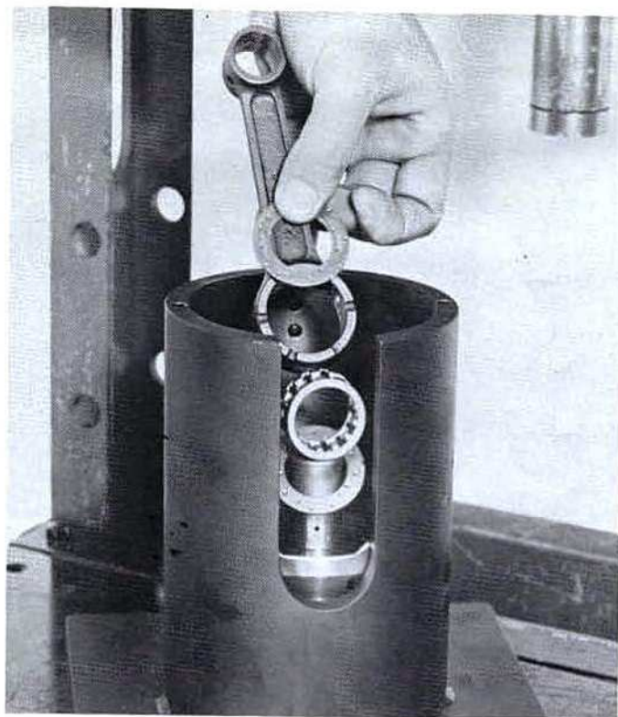
6 Install new connecting rod assembly, thrust washer—big end bearing—con rod—thrust washer. As shown. NOTE: Pack big end bearing with a suitable hi-temp grease.
