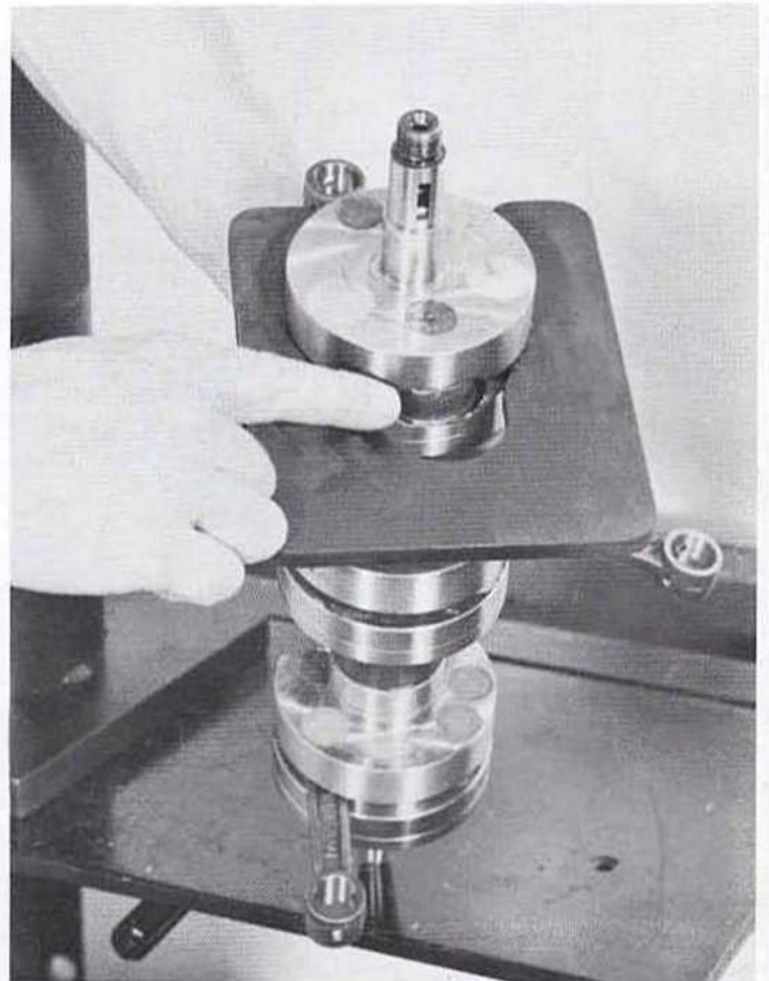
4 Place the flywheel support plate (tool S) between the flywheels of the left-hand crank assembly. (Position the support plate so that the big end of the connecting rod is at the closed end of the rod access slot in the support plate.)
