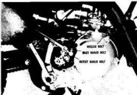
Start the engine and then pull open the pump control lever to bleed the pump and prime the engine with oil. When the exhaust starts smoking heavily, release the lever and seat the cable nipple in the lever. CAUTION: If the engine does not start smoking, or if bubbles are present in the oil pressure line, check for blockage or loose connections.
