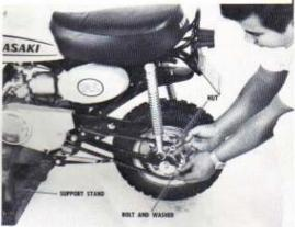
Check for any loose parts inside the brake panel and the brake drum, and then install the front brake panel in the front wheel drum. The short spacer is used next to the brake panel, SAFETY NOTE: Loose parts inside the brake assembly could cause the front wheel to lock, resulting in the loss of control.
