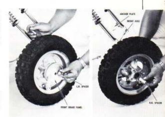
Swing the brake panel so that it lines up with the fork tube anchor tab. Insert the bolt from inside, and then secure it with the large flat washer, lockwasher and nut. Tighten the axle nut at this time.
