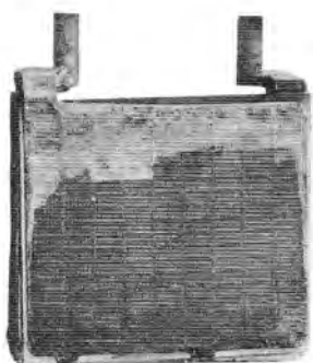
Fig. 15 Plate with sulfation by short electrolyte
